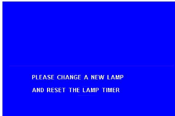
Figure 15 Lamp replacement warning signal
