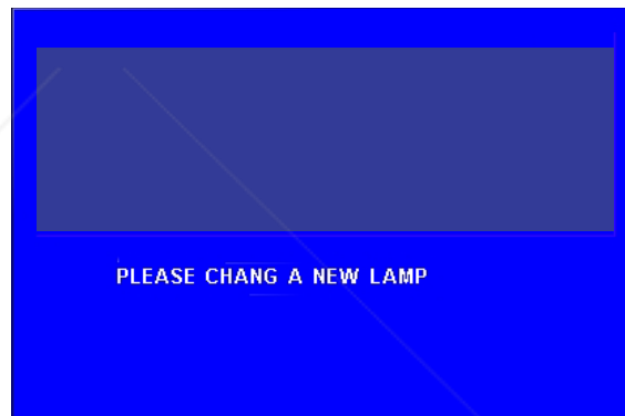
Figure 17 Lamp replacement warning signal
