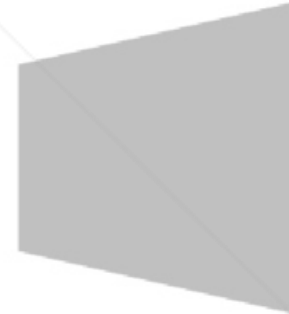
From the projector, the image path is shorter along the left side.
