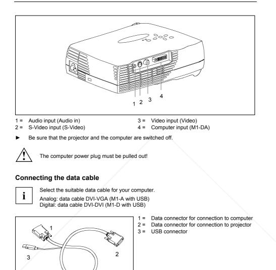
Connect the connector (1) of the data cable to the active monitor port on the computer and secure the plug-in connection by tightening the safety screws.
