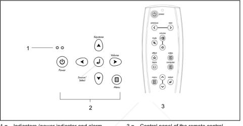
1 = Indicators (power indicator and alarm indicator) 3 = Control panel of the remote control
