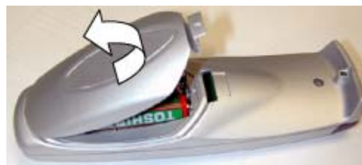
Image 8-2 Battery cover removal
