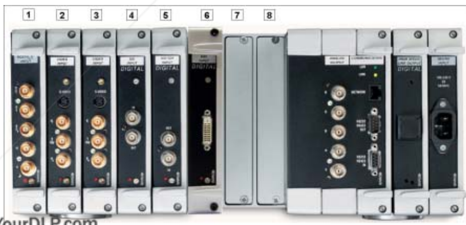
Image 7-20 Input modules overview
