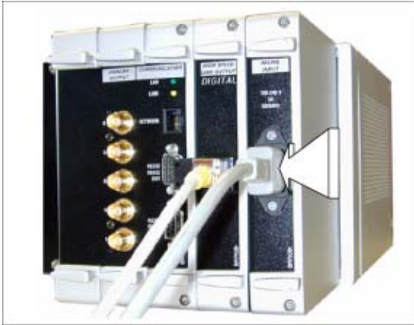
Image 7-5 Insertion of the power plug
