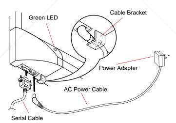
Plug the other end into your PC's serial port (if necessary, use the 9-to-25-pin adapter) and tighten the screws.
