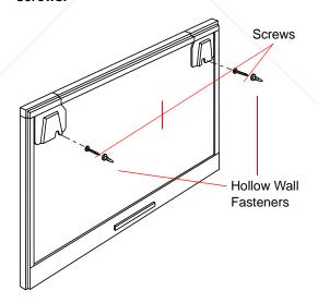
Hang the whiteboard on the screws using the slots at the top corners in back.
