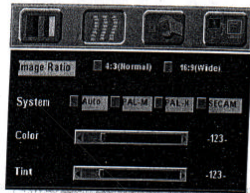
Figure 24 Image sub-page – Only available when the input signal is from video, S-video
