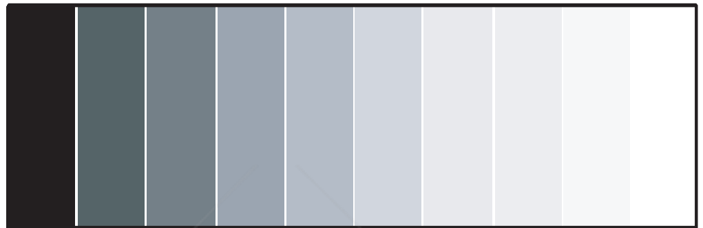
Figure 4-3. Typical Gray Bar Pattern for Adjusting Contrast
