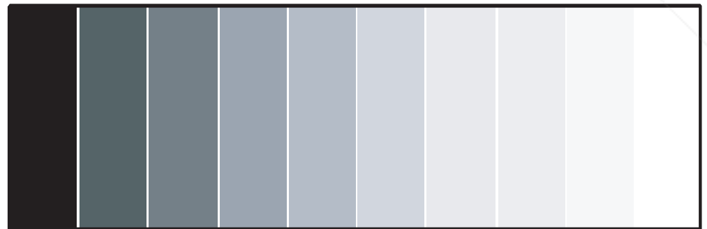
Figure 4-3. Typical Gray Bar Pattern for Adjusting Contrast
